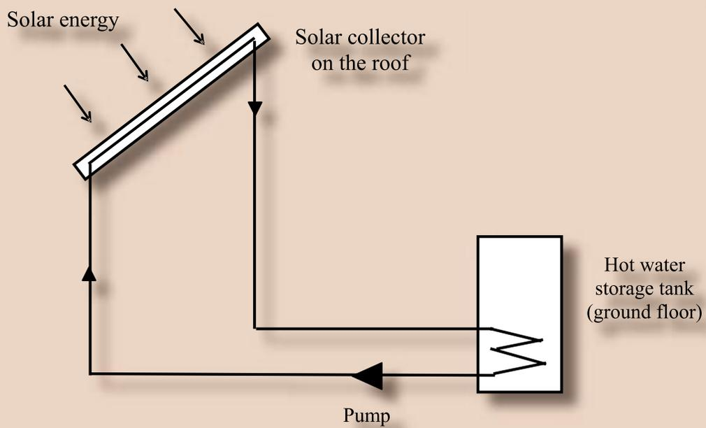
**Figure 3.2 Typical solar domestic water heater with pump (schematically)**
