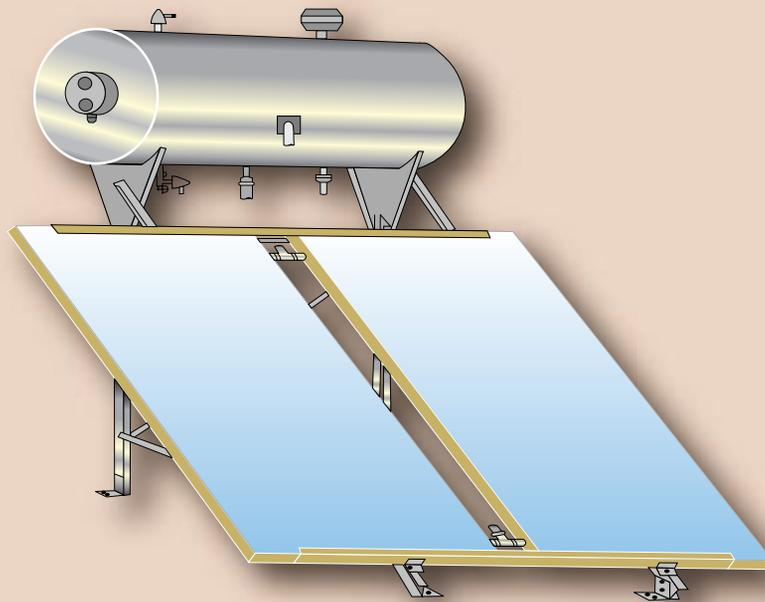
**Figure 3.1 Typical solar domestic water heater of thermosiphon type**
