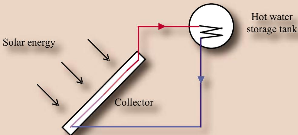
**Figure 6.1 Schematic presentation of a thermosiphon system**
