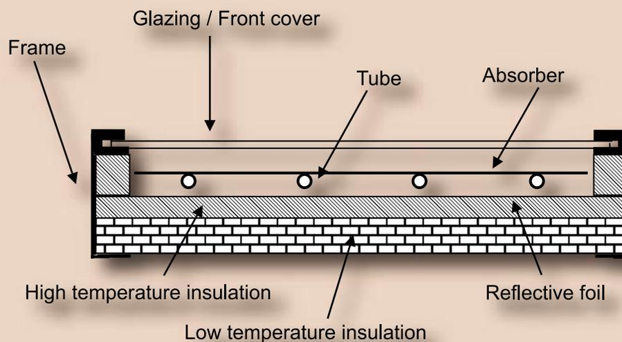
**Figure 4.1 Typical cross section of a glazed liquid heating solar collector**
