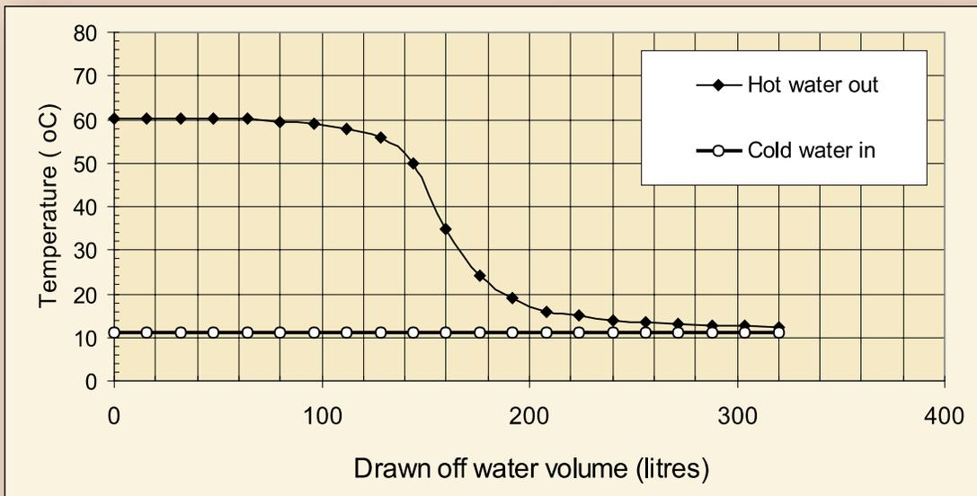
**Figure 11.1 Temperature of the hot water of a solar domestic hot water system with a tank volume of 160 litres (thermosiphon type)**
