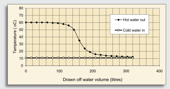
Figure 4.1: Temperature of the hot water of a solar domestic hot water system with a tank of 160 litres
