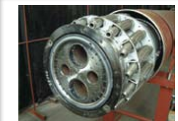
M.A.S. Burner for standard fuels, waste fuel oils and solid secondary fuels. Source: Unitherm Cemcon
