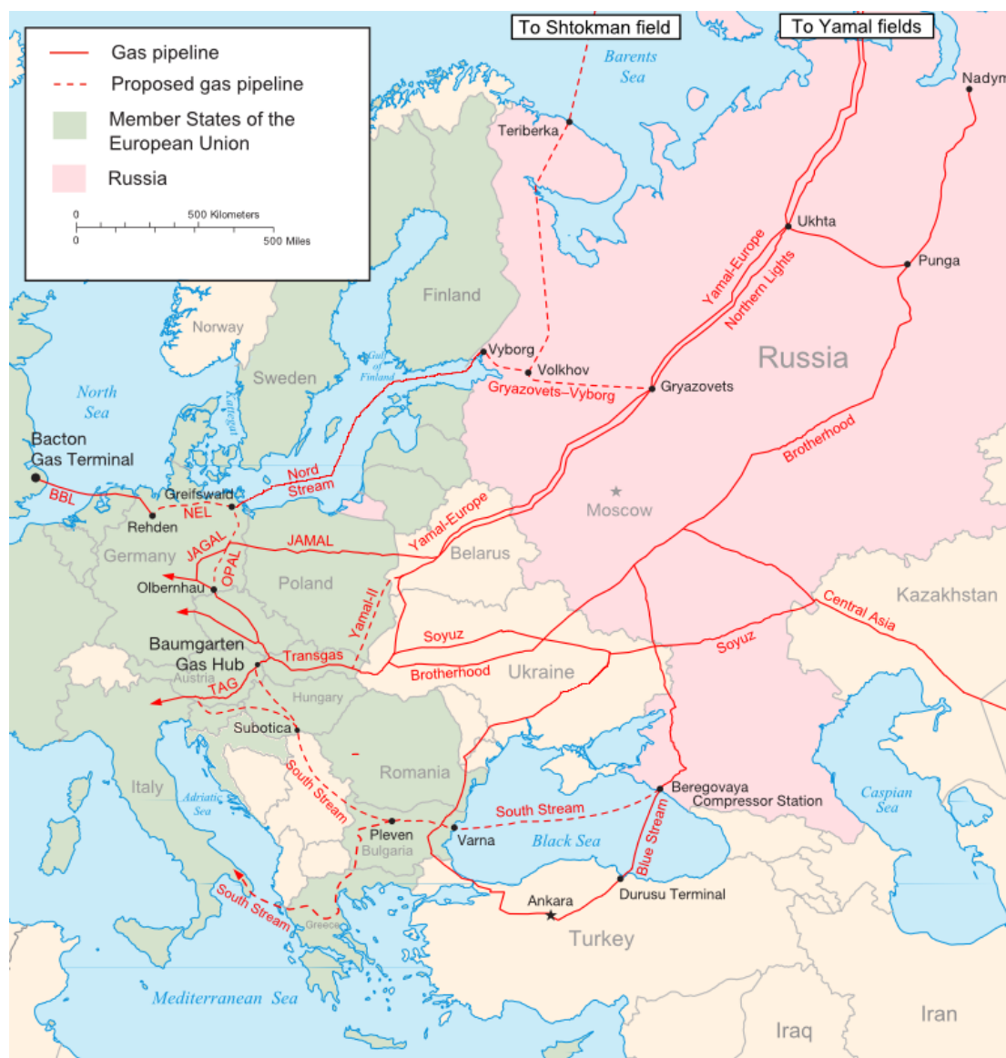
Figure 3.32: Map of major Russian natural gas pipelines arriving to Europe (Source: Wikipedia)
