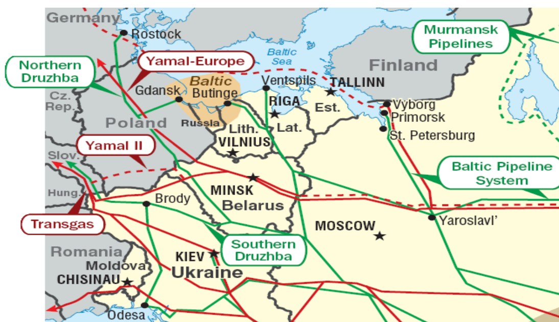
Figure 3.17: The Baltic Pipeline System. Gas pipelines are shown in red colour, oil pipelines in green and the dashed line shows the planned pipelines. (source: EIA)
